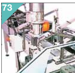
73 000935-01 SIRIO 370 AF-NC SLB6 VELOX 350 AF-NC SLB6 Guide superiori per diametri fino a 10mm. Device to load bars up to 10 mm.
